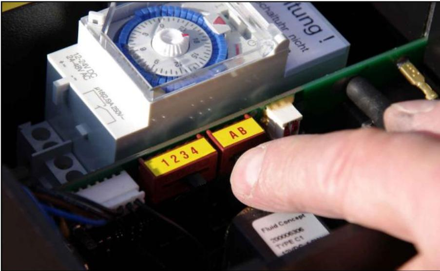
To set up the volume of the unit use the A/B switch.
