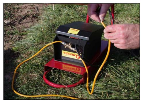
Remove the propane nozzle which is plugged into the gas hose (Gh-2) which runs away from the electronic unit (solenoid valve side arrow front).
