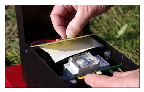
Open the lid from the electronic unit (108510). Lift the battery contact board and remove the paper strip to contact the batteries with the board. After removing the paper strip press the battery contact board back down to close it.
