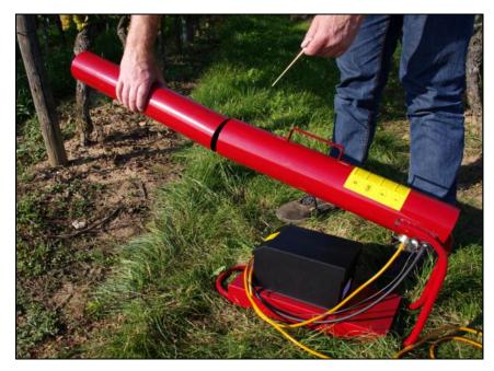
Slide the sound tube into the shot frame and secure it with the lock pin (130012). See next page for sound tube settings.
