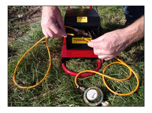
Now connect the gas hose (Gh-1) which goes away from the electronic unit (solenoid valve side arrow end) with the gas hose from the gas regulator (101660).
