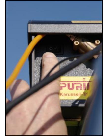
Open the valve of the gas bottle and switch on the unit.
