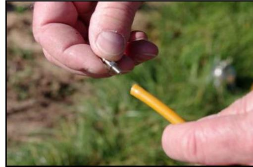
Remove the propane nozzle which is plugged into the gas hose (Gh-2) which runs away from the electronic unit.
