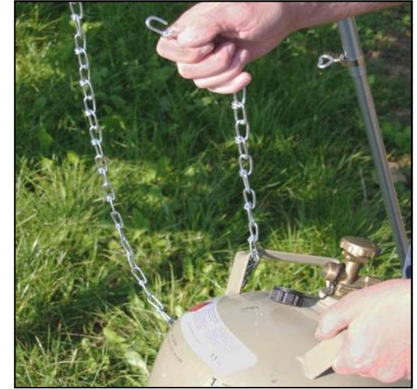
Hang one side of the chain (102080) with the sharp end of the hook pointing out of the bearing block. Move the chain through the handle of the bottle and attach the other end of the chain also to the bearing block (sharp end outside!)
